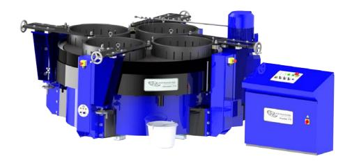
The Lapmaster Model 72 is equipped with a 1829mm diameter lap plate. This is manufactured from Grade 300 grey cast iron to ISO 185(2005). It consists of individual segments bolted to a support plate.
